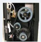
**Vertical tensioned belt** provides extended life and reduced maintenance costs by eliminating multiple belts that stretch at different rates.
